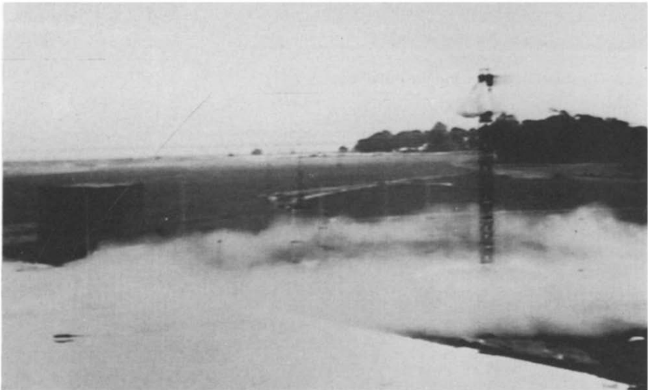
Fig.20. Trial 026: Cloud passing around the obstruction in a low wind.
