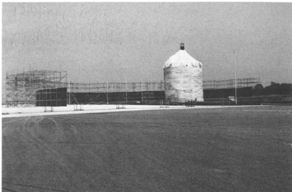
Fig.2. Obstruction 1 : 5 m high impermeable barrier.
