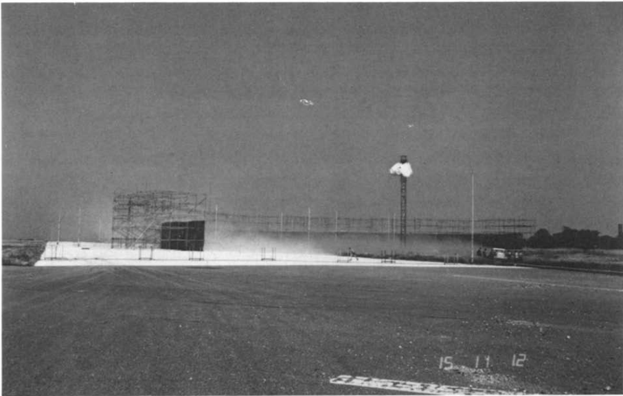
Fig.4(a). Trial 020: Largely unblocked cloud advection in presence of 5 m barrier.
